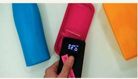
Figure 2: Plastic scanner scanning plastic product
