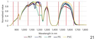
Figure 2.5: Spectroscopy plot, with PlasticScanner wavelengths (red lines).
