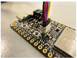
3.31 Qwiic connector on an ESP32 Feather
