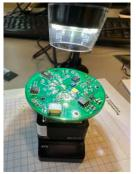
colour sensor from Adafruit [73], I2C-supported and the NAU7802 ADC design by Adafruit [74]. To be able to fit all components into the circular design, it was decided to switch the size of passive components (resistors and capacitors) from a 1206 to a 0603 footprint. This change makes it harder, but still possible, to hand solder the components, but made it pos-
