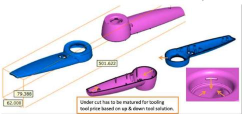
3.40 Mould layout sketch from manufacturer, with markings of mould insert and pull-outdirection
